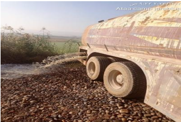
Figure 11: Desludging Tanker Discharging the Wastewater to the Valley
